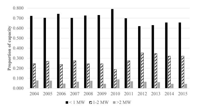
Figure 3: Proportion of the Time that a 3.5-MW Capacity Alberta Aggregated Wind Turbine would Produce less than 1 MW, 1-2 MW and more than 2 MW of Electricity during a Year, 2004-2015
